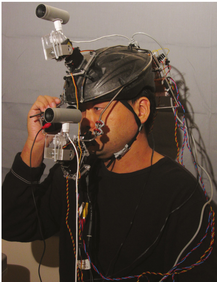
Imagen 5. Jeong Han Kim, BirdMan's Vertical Eye Tracking System, 2006-2008. Wearable perception device (MaxMAP/Jitter, three cameras, four servomotors, PIC-microcontroller), variable size. LMCC, New York, NY, U.S. & Seoul, Korea.
