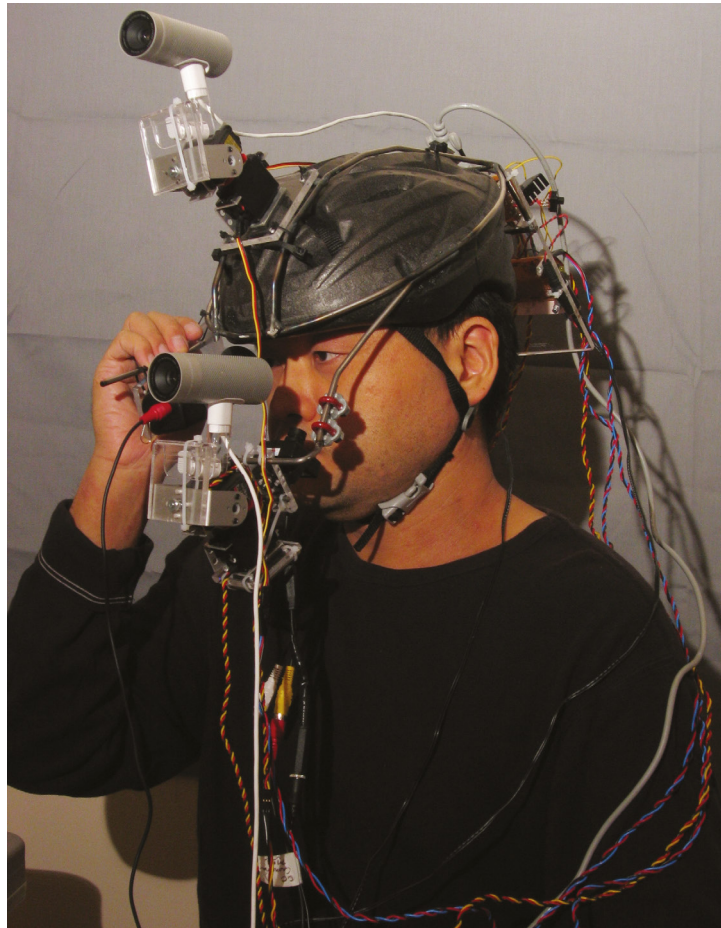
Image 5. Jeong Han Kim, BirdMan's Vertical Eye Tracking System, 2006-2008. Wearable perception device (MaxMAP/Jitter, three cameras, four servomotors, PIC-microcontroller), variable size. LMCC, New York, NY, U.S. & Seoul, Korea.
